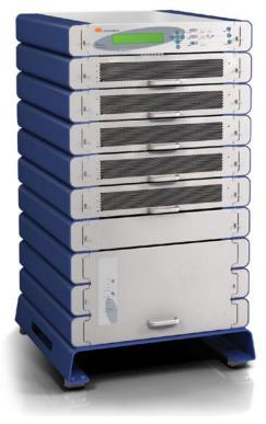
The **Gamatronic Power+ M50** is a parallel redundant modular UPS capable of scaling from 10kVA to 50kVA. Comprised of one to five 10kVA/8kW UPS modules, as well as a system controller, a 50kVA static switch, and a distribution block, the system easily grows with your requirements.
