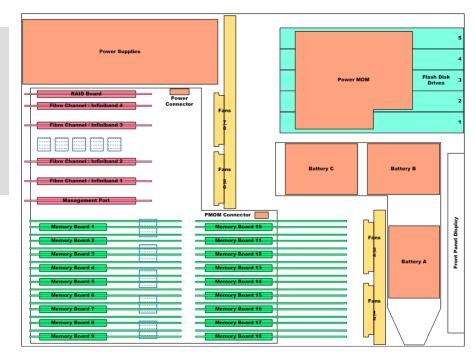
DDR-RAM memory, the primary storage media, fill the back of the unit. The front contains backup batteries, backup mechanical drives, and a front panel user interface.
