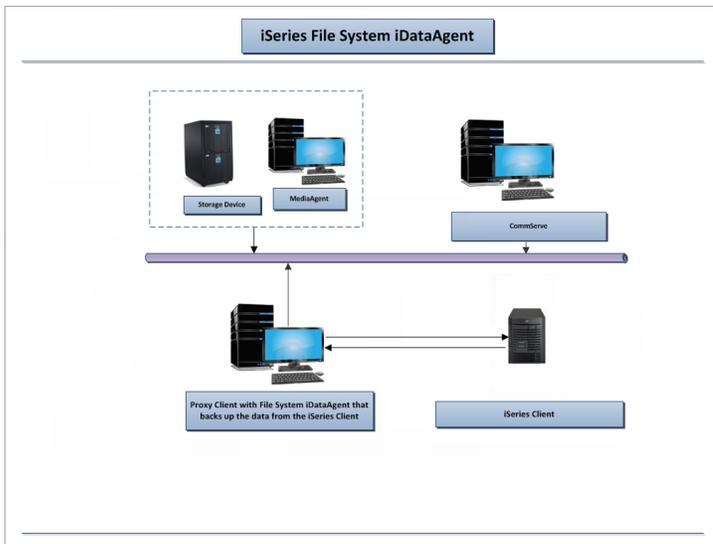
Alternative configuration with MediaAgent and Proxy Client on the same computer:
